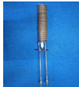
Gambar 3. Foto Kondensator Dummy Tipe Helical Coil Diameter 1/4" Panjang 6,7 meter
