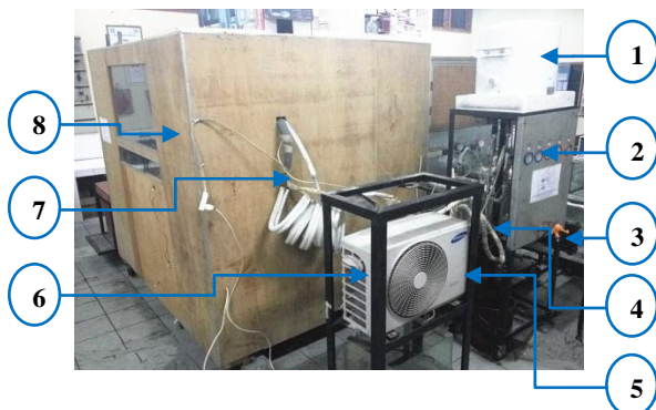
Gambar 2. Foto Air Conditioning Hibrida
